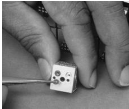
Figure 5.12 DH200 Transducer O-Ring Replacement
